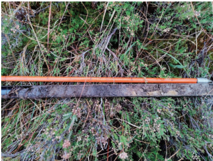
Photo 2 Example of a peat core showing a distinct layer of gritty silt.
