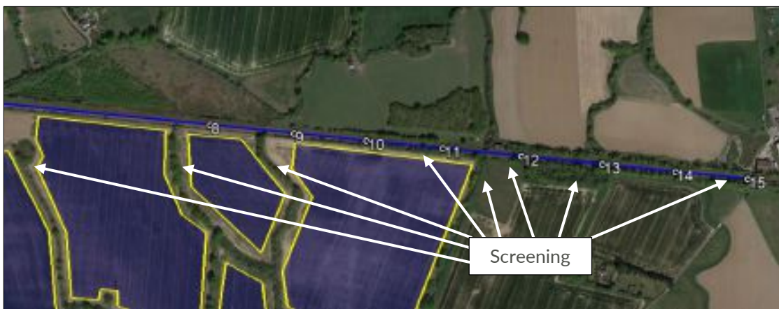
Figure 26 - Identified screening for the railway receptors
