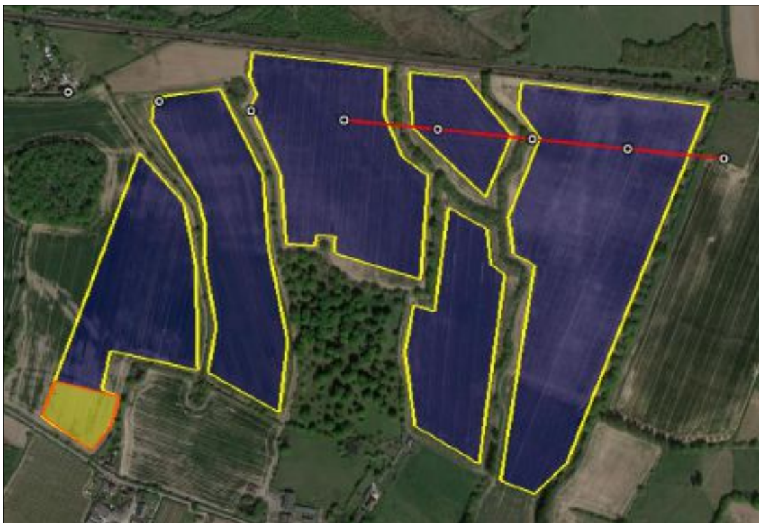
Figure 15 – Sections of the proposed development which will generate yellow glare and relative section of the approach path affected
