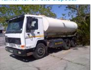
Where it has not been possible to adequately treat construction site runoff there remains the option to pump the runoff out to a tanker for disposal off-site at a suitably licensed waste facility.
